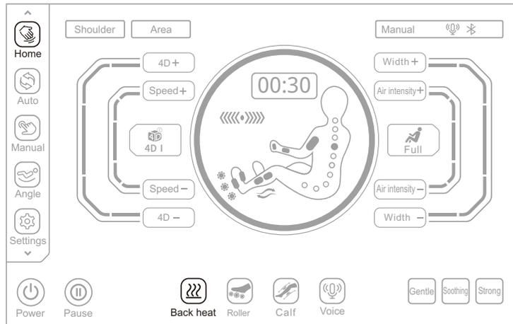
In the "Home" interface, click the "Roll" button to turn on or off the foot roller massage function, with three adjustable speeds.
