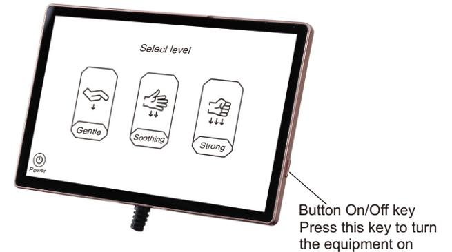
2. After the system is started, select the massage intensity by clicking on any one of the Gentle , Comfort or Strong keys on the remote controller to turn on the massage chair and enter the lying state. If it is not selected within 5 minutes, the massage chair will turn off automatically.
