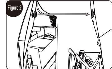
3. First, lift and tilt the front of the armrest, then place the rollers at the rear end of the armrest into the corresponding slots on the side of the capsule (Figure 2), push the armrest towards the upper rear end, and push the roller to the limit position of the slot. (Figure 3)
