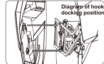
4. Press the front end of the armrest down, and hang the hook position on the armrest to the pipe fittings of the steel frame assembly. The front side screw position of the armrest is aligned with the steel frame assembly and exposed, which means it is assembled in place. (Figure 4) Finally, lock with 2 M5 screws. (Figure 5)
