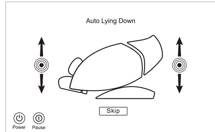
3. For automatic angular adjustment, select the automatic program, then the massage chair will be automatically adjusted to zero-gravity angle, and wait until its adjustment is completed. To skip a step, press the skip key to go directly to the next step.
